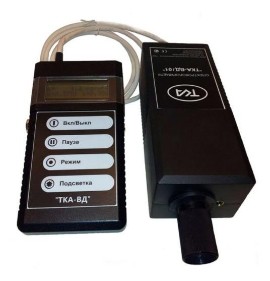
The device consists of one 01-optoelectronic unit (input objective Ø21 with a coated lens) and a signal processing unit, interconnected by a flexible multicore cable. In this case, measurements are made only of self-luminous overhead method and cinema screens in brightness mode. A device with a linear detector with a fixed position of the diffraction grating has no moving parts, which makes it possible to simultaneously record a relatively wide visible spectral region with imaging.
