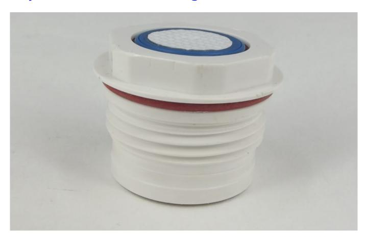
The replaceable measuring module is a measuring element that is used in the "GastroTest" device. The main element of the module is an electrochemical ammonia sensor (electrochemical sensor). The service life of a replaceable module is 12 months from the date of sale of the device, but no more than 600 tests. At the end of the service life, it must be replaced. Module weight is 17 g, overall dimensions  $-\emptyset$  34 mm and height 26 mm.
